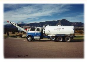
arker Ag currently operates a large fleet of semi tankers for transporting liquid biosolids in large volumes. Each tanker holds about 6,500 gallons. Small volumes are managed using straight trucks with 2,500 to 4,000 gallons of capacity. The number of loads removed range from one load per week to as many as 50 loads per day.
